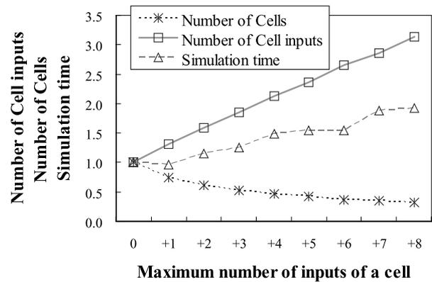
Fig. 12 Relation between the maximum number of cell inputs and simulation time.
