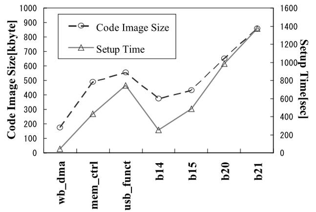
Fig. 17 The code image size for LCC and the simulation setup time.
