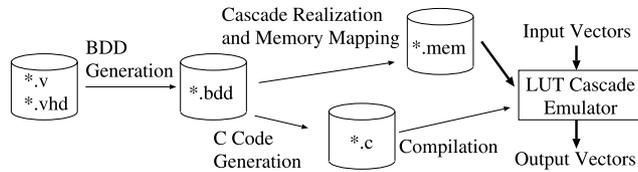
Fig. 11 The logic simulation system using LUT cascade emulator.
