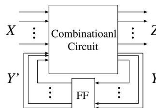
Fig. 1 A model for a sequential circuit.
